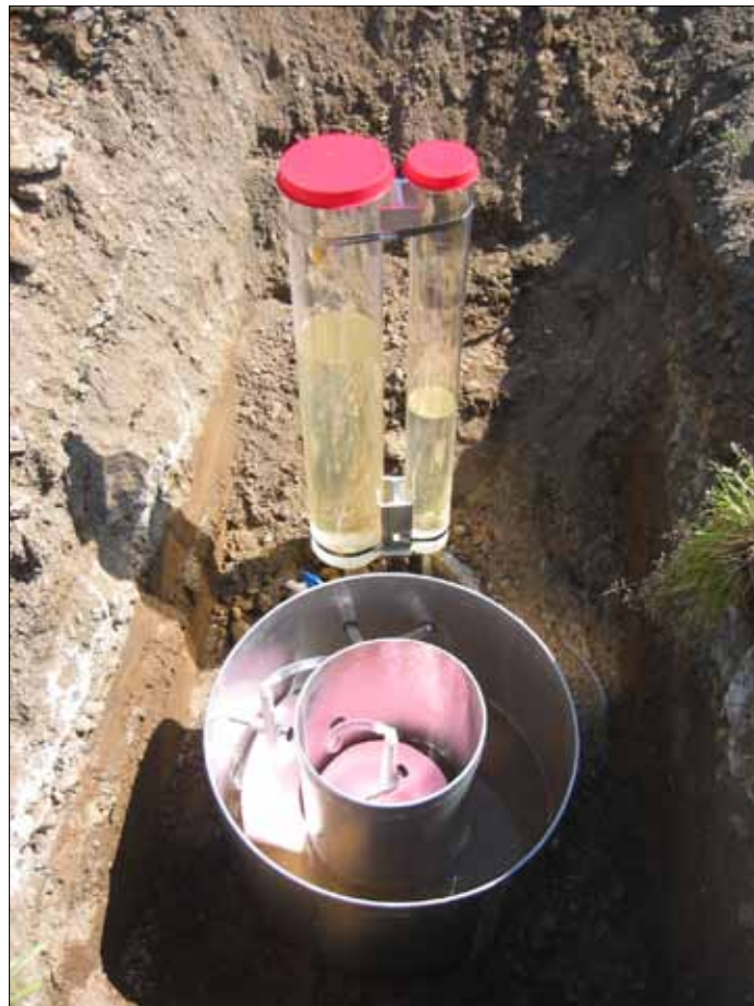
Double-ring infiltrometer with optional measuring beakers.
