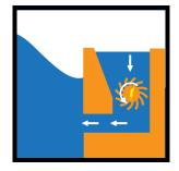
A collector funnels waves over the top of the structure and into one of the device's reservoirs, positioned below the waterline. The water is then run back out to sea through one or more turbines. As the water spins the turbine rotors, electric current is generated. This device can be found on shore or in open ocean.
