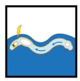
The bulge wave is a rubber tube filled with water. The passing wave causes pressure variations, which create a bulge within the tube. Energy is gathered as the bulge moves, along with the wave, toward a turbine in the bow of the tube.
