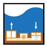
A pressure differential is created in the device as waves cause sea level to change as they pass. The vertical motion caused by the differential drives a fluid pump that creates mechanical energy.
