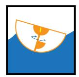
A rotating mass device heaves and sways in the waves, causing a gyroscope or weight to rotate within. The movement is attached to a generator inside the device, which produces energy.
