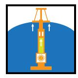
The point absorber is a floating structure that captures energy from the vertical motion of the waves. This up-anddown motion of the device drives generators that create an electric current.
