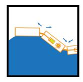
The wave attenuator is a multi-segmented device that captures energy as the motion of the wave causes it to flex where the segments connect. This movement then drives hydraulic pumps or generators.
