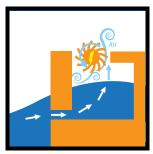
These are partially submerged structures that house a column of air above a column of water. Waves are funneled into the structure below the water line, forcing the water column to rise and fall like a piston. This movement both pressurizes and depressurizes the air column, moving a turbine with the resulting "push/pull" force.
