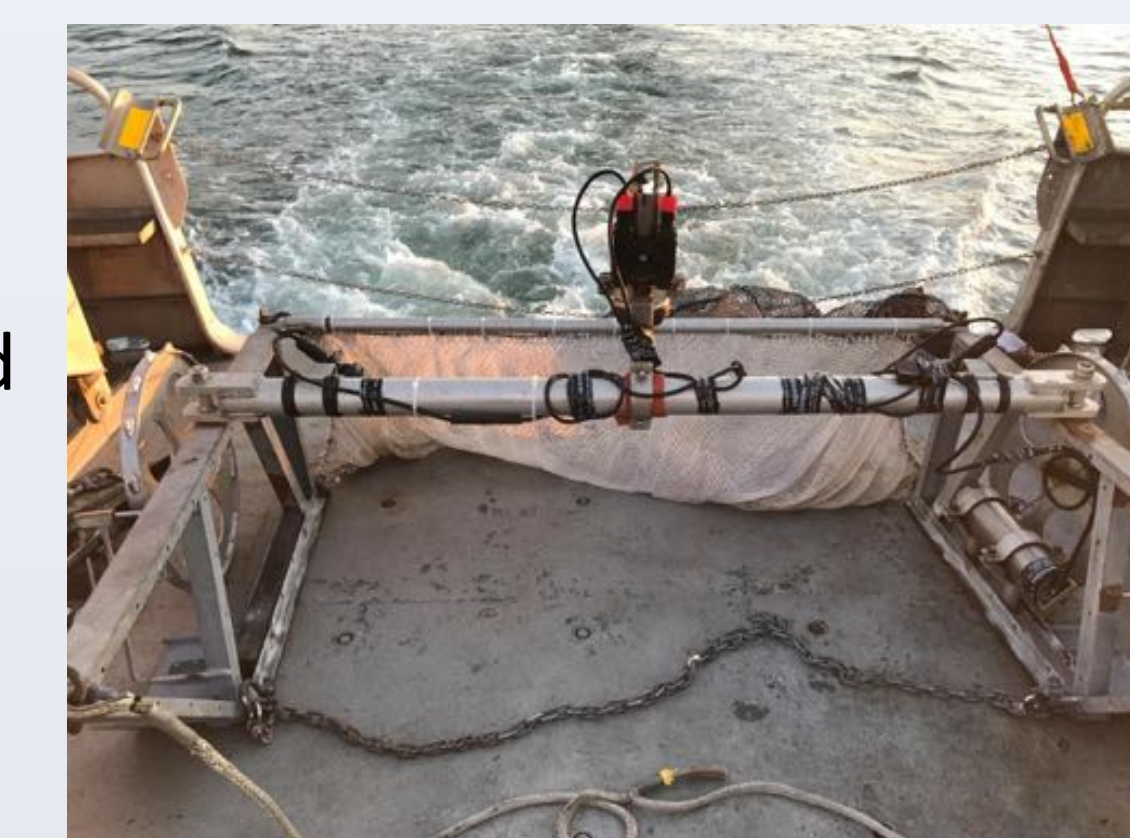
Figure 4. Two meter wide beam trawl used in NH line study.
