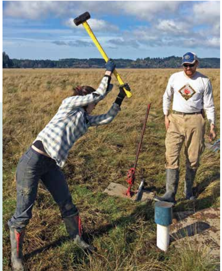
Graduate students take turns pounding a soil corer into the Alsea Bay high marsh. The work was part of research funded from 2016 to 2018 by Oregon Sea Grant. (Photo by Rob Wheatcroft)
