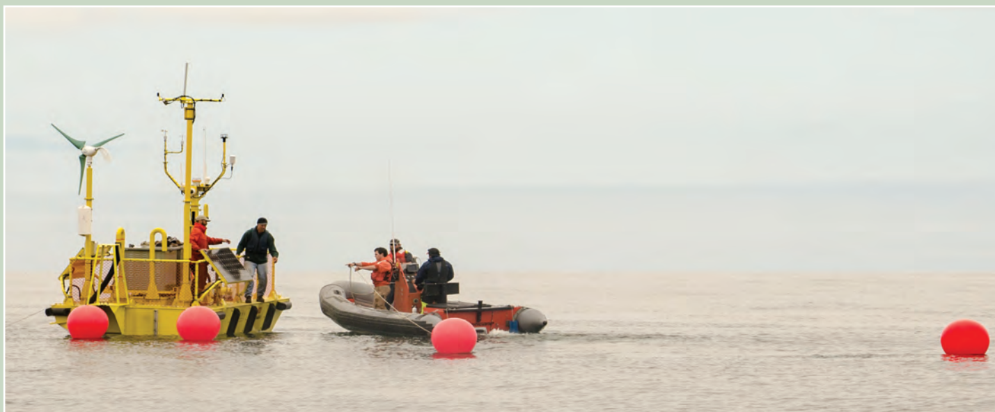
Oregon State University researchers set up the wave energy testing buoy Ocean Sentinel near Newport, Oregon.
