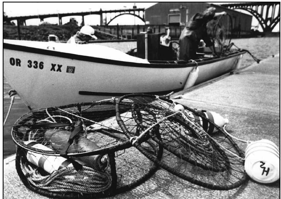
Figure 1 A crab trap (left) is bulkier than a crab ring net (right), but you can leave the trap unattended longer without fear of losing your crabs.
