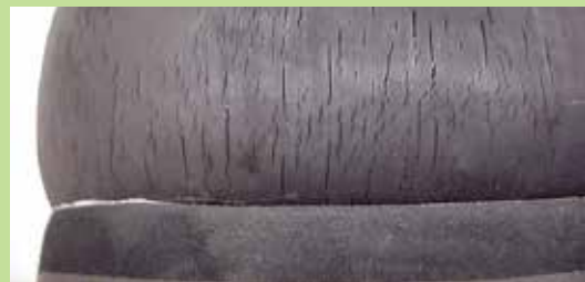
The toe of this rubber wader boot has cracked after being exposed to repeated applications of benzethonium chloride. (Photo by Robert Hosea.)
