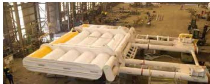
This style of device harnesses wave energy directly from the surging and swelling motion of waves. It uses the oscillation between a float, flap, or membrane and a fixed point. That movement creates a usable form of mechanical energy. Similar devices are also being developed that utilize pitching, heaving, and swaying motions.
