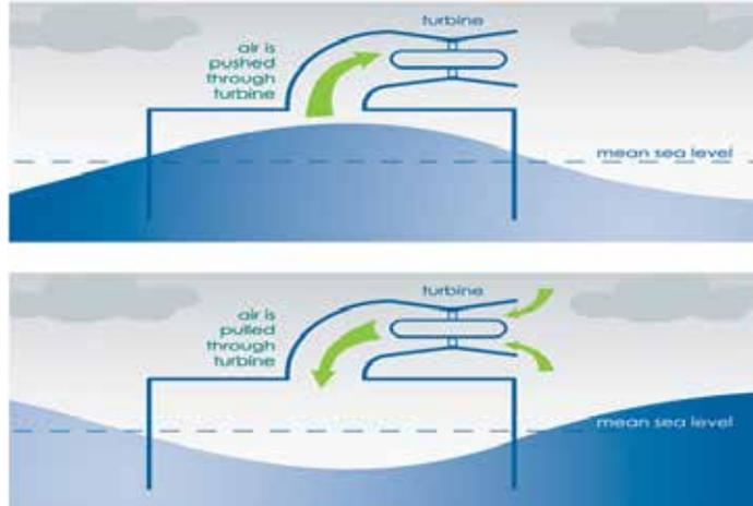
These are partially submerged structures that house a column of air above a column of water. Waves are then funneled into the structure below the waterline, forcing the water column to
