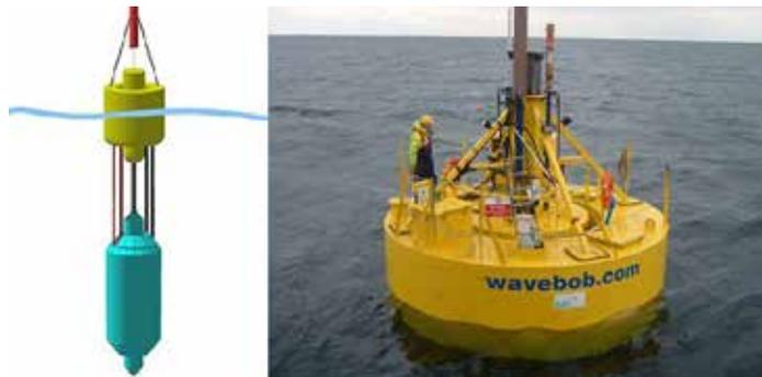
The point absorber is a floating structure that captures energy from the vertical motion of the waves. This up-and-down motion of the device drives generators that create an electric current.
