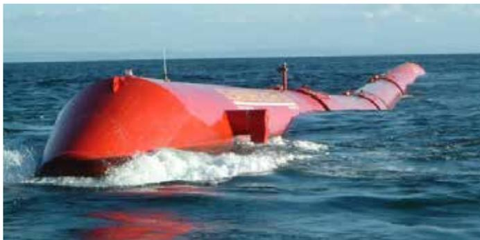
This device is long and multi-segmented and floats on the surface. The attenuator is anchored in place with a mooring line and positioned perpendicularly to incoming waves. Some attenuators tap only the heave (vertical motion); others tap both heave and surge. The device captures energy as the motion of the wave causes it to flex where the segments connect. This movement then drives hydraulic pumps or generators.
