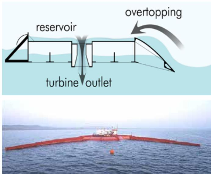
The overtopping device generally is constructed on shore or on a levee. There is a collector that funnels waves over the top of the structure and into one of the device's reservoirs positioned below the waterline. The water is then run back out to sea through one or more turbines. As the water spins the turbine rotors, electric current is generated.
